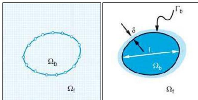
figura 4.20- Confronto tra immersed boundary IB (sx) e body conformal (dx)
