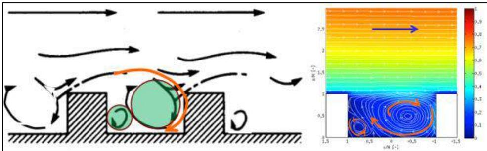
figura 1.15 - wake interference flow  $1.5 < \frac{H}{d} < 2.5$
