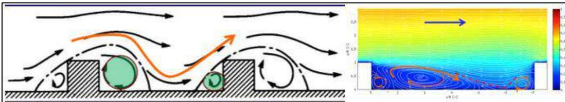
figura 1.16 - isolated roughness flow  $\frac{H}{d} > 2.5$
