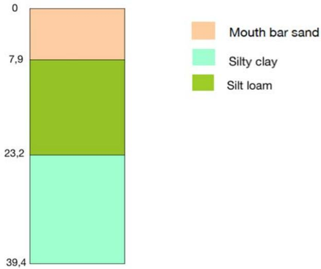
**Figure 43:** Decompacted sedimentary columns representative of marine environment in Krishna delta.
