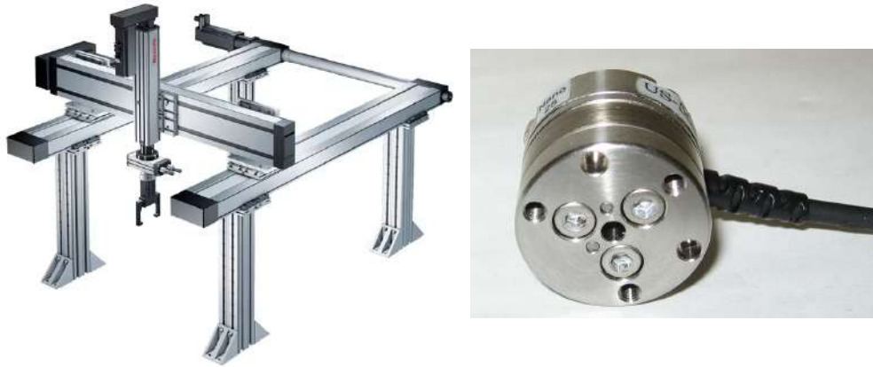
Figure 3.13: On the left an example of Cartesian robot; on the right the ATI Nano Series 6-axis force/torque sensor.
