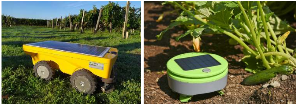
Figure 2.15: On the left the completely autonomous mobile robot for precisely controlling soil grassing proposed by VITIROVER Solutions; on the right Tertill Weeding Robot.
