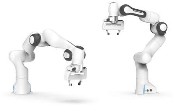
Figure 3.1: The Franka Emika Panda robotic arm equipped with the Franka Hand 2-fingers gripper.
