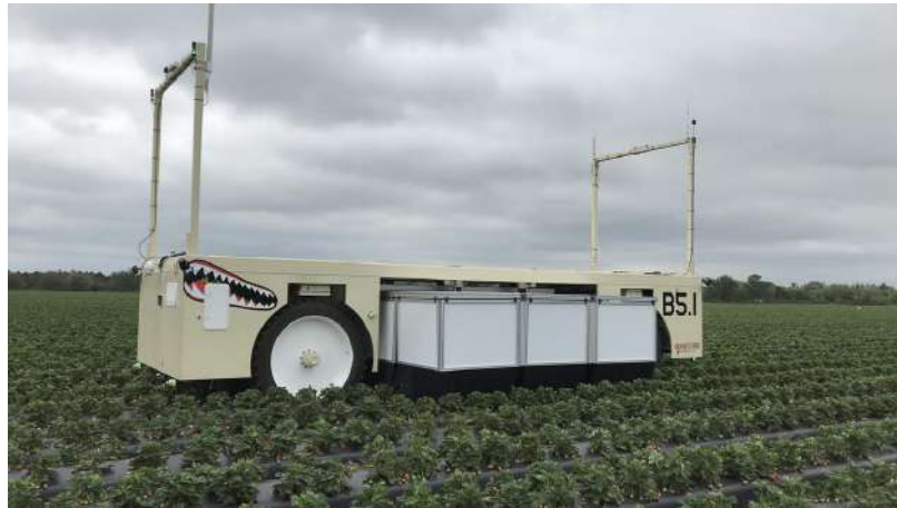
Figure 2.17: Harvest CROO Robotics Berry 5 fruit picking robot.
