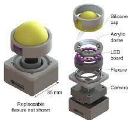
Figure 2.27: A rendering of the Visiflex [18] tactile sensor and its exploded view.
