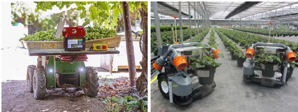
Figure 2.18: On the left Augean Robotics' Burro self-driving robot; on the right Harvest Automation's HV-100 robot.
