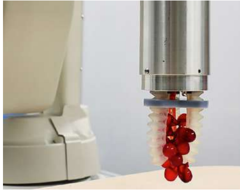
Figure 2.8: Cambridge Consultants' Hank soft gripper.
