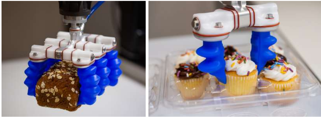
Figure 1.2: Soft Robotics' mGrip: a modular gripping system that enables reliable, high-speed picking of traditionally hard-to-grasp single items.
