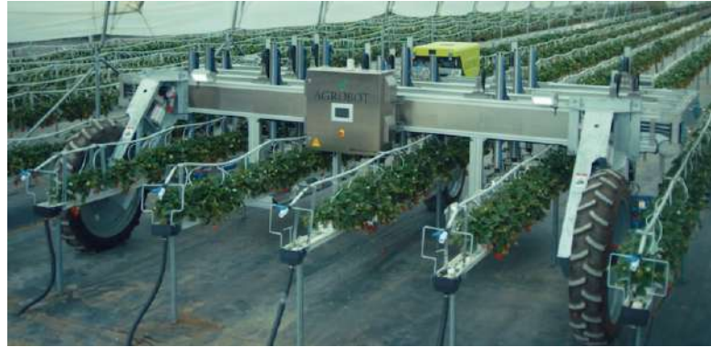
Figure 2.16: Agrobot E-Series stainless steel and military-grade aluminum robot.
