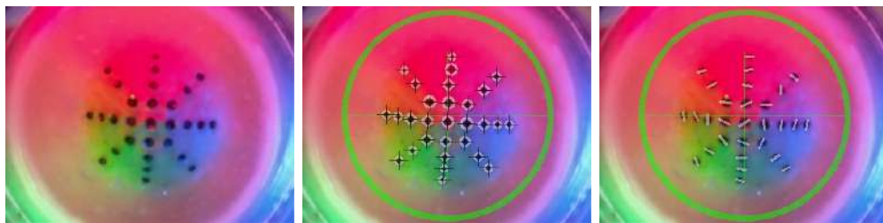
Figure 3.21: Left: the raw frame when a normal displacement of 10mm is caused by the external force. Center: the frame after marker detection, fitting ellipses. Right: the frame after marker detection fitting circles.
