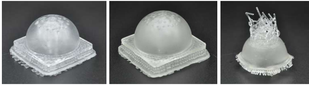
Figure 3.3: From left to right: the just printed dome; the washed dome; how the washed dome presents on the inside.
