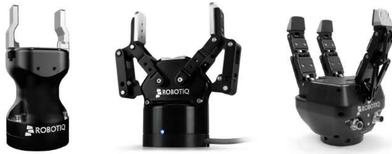
Figure 2.2: From left to right: ROBOTIQ Hand-E Adaptive Gripper, 2F-85 Gripper and 3-Finger Adaptive Robot Gripper.
