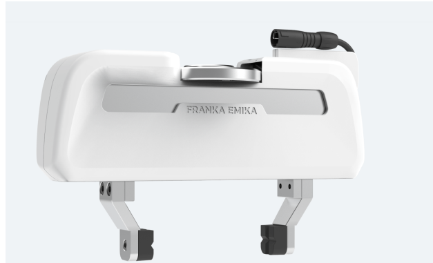
Figure 3.15: Original Franka Emika Hand gripper.
