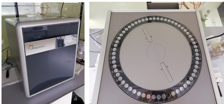
Figure 13 Vario MACRO Cube employed for the elemental analysis and an upper view of the charging disc
