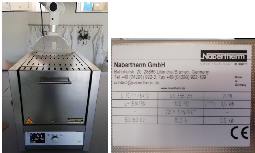
Figure 7 Picture of the muffle furnace used for the stabilization process and its technical specifications
