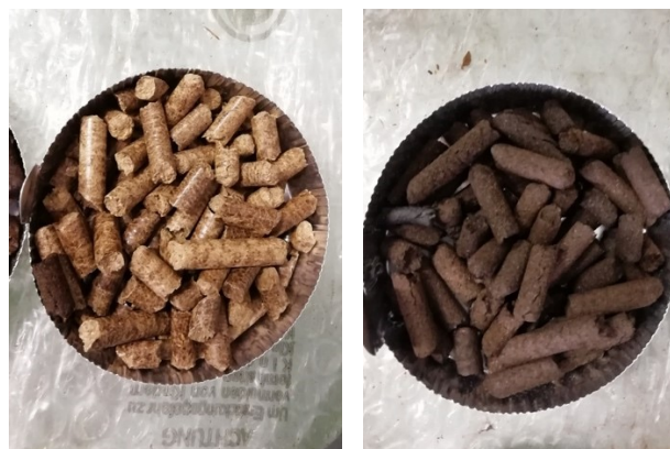
Figure 45 Samples of a standard pellet and a torrefied pellet
