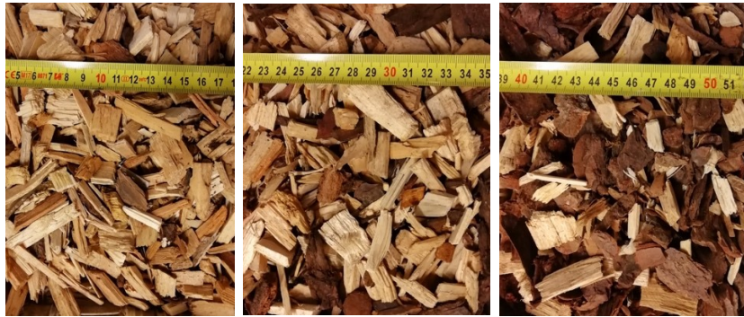
Figure 25 From left to right, samples of wood fraction without bark, 30% blend, 80% blend
