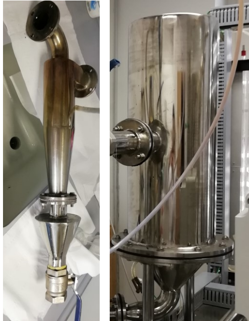
Figure 20 On the left side, the cyclone separator during maintenance operations, on the right figure, the fabric filter container
