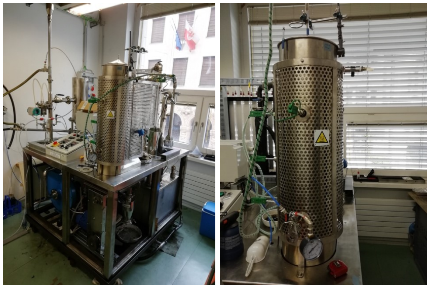
Figure 19 Picture of the open top gasifier in Free University of Bolzano and on the right, the main reactor
