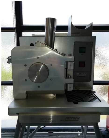
Figure 8 Cutting mill used for the bark pretreatment
