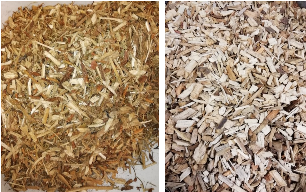
Figure 3 On the left a forestry woodchip, on the right an higher quality woodchip
