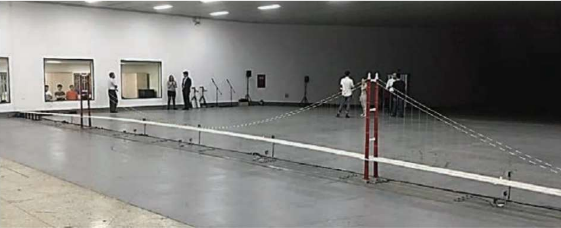
Figure 4: 1:190 scale full aeroelastic model of the 1915 Çanakkale Bridge at the RCWE boundary layer wind tunnel.
