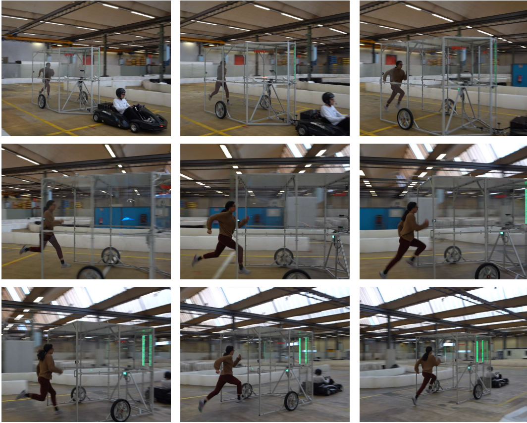
Figure 4.8: Sequence of images taken from a video, showing a tracking regulated with MPC
